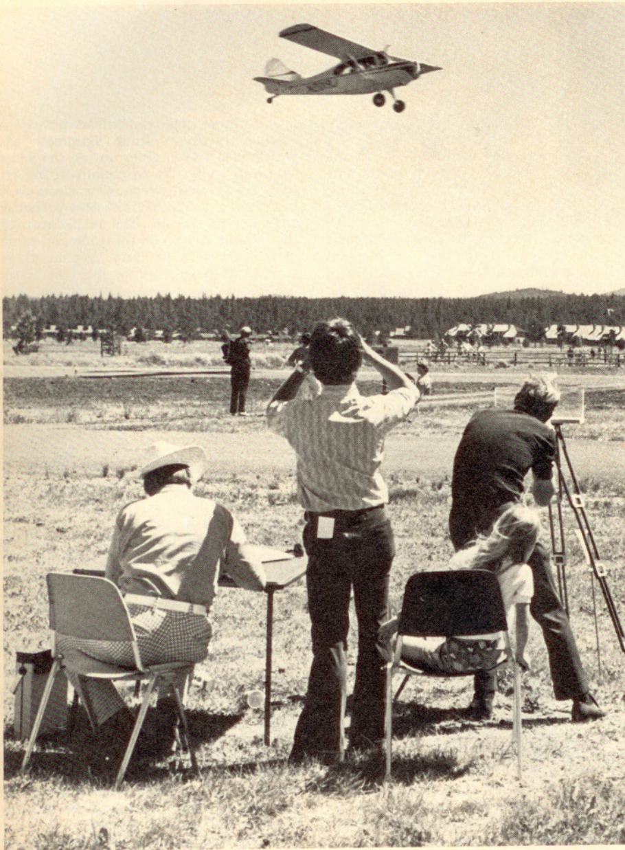
Thedolite "scores" pilots' abilities to cross imaginary 50-foot obstacles on high-density altitude takeoffs. Most fell short of their expectations.
